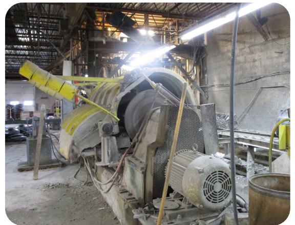
Tank is centrifugally spun at an RPM and length of time specific to the size of the tank
