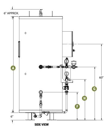
Note: Welded Steel Skid option adds 9" to overall height of unit
