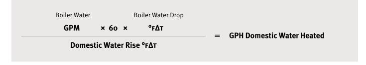
**Note:** A minimum  $10^{\circ}F$  differential ( $\Delta T$ ) between the exiting boiler water temperature and the exiting domestic hot water temperature is required to maintain efficient heat transfer rates. For detailed information regarding the heating coil, please reference the Hubbell brochure titled "Hubbell Heating Coils".
