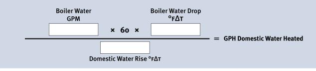
**Note:** A minimum  $10^{\circ}F$  differential ( $\Delta T$ ) between the exiting boiler water temperature and the exiting domestic hot water temperature is required to maintain efficient heat transfer rates.
