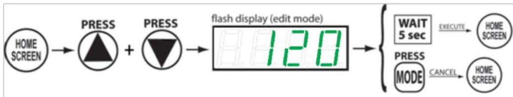
To access the options menu, from the home screen, press and hold the **MODE** button until the display reads “diF” (differential), this is the first selection in the options menu.
