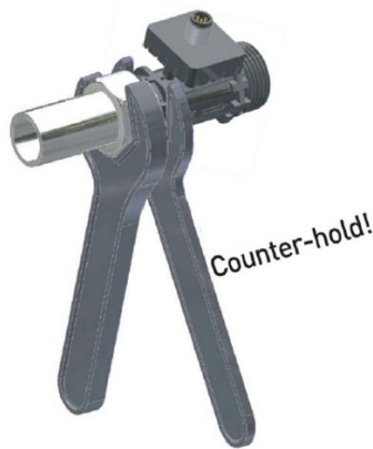
Figure 4. Use a Backup wrench to prevent the vortex flow meter from rotating.
