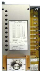
Solid State Staging Controller
