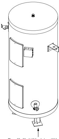
Three 2" x 2" x 1/4" Angle Legs With 4 x 4" x 1/4" Base Pads and 5/8" Diameter Bolt Holes on 15" Diameter **Bolt Circle for Deck Mounting**
