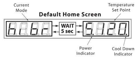
By default, the Hubbell Hot Water Heat Pump comes programmed with a temperature setpoint of 120°F and set to hybrid mode ("hibr").
