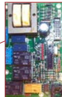
Electronic control module integrates all control functions into one component
